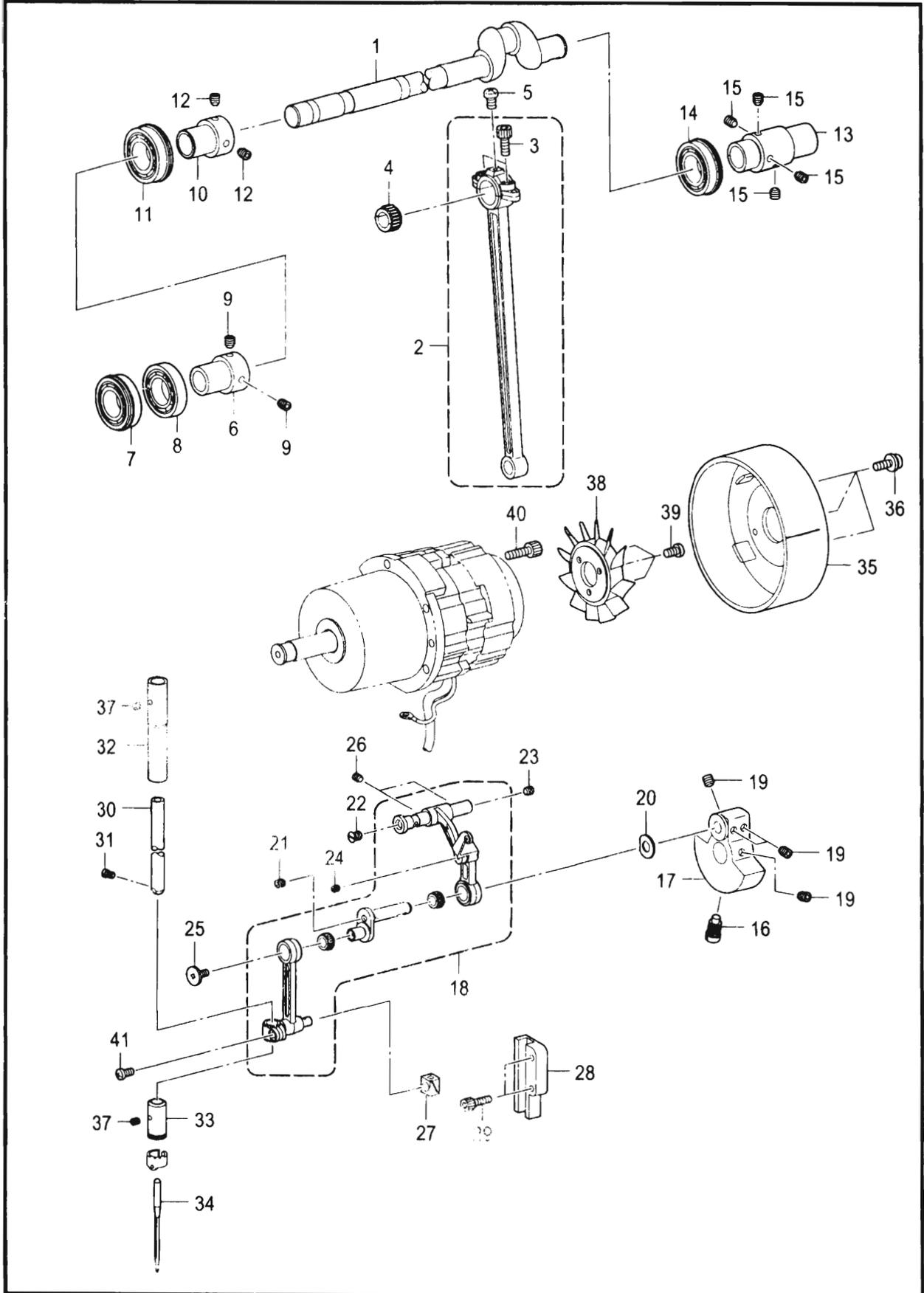
B. 上轴 · 针杆装置 / Upper shaft and needle bar mechanism
