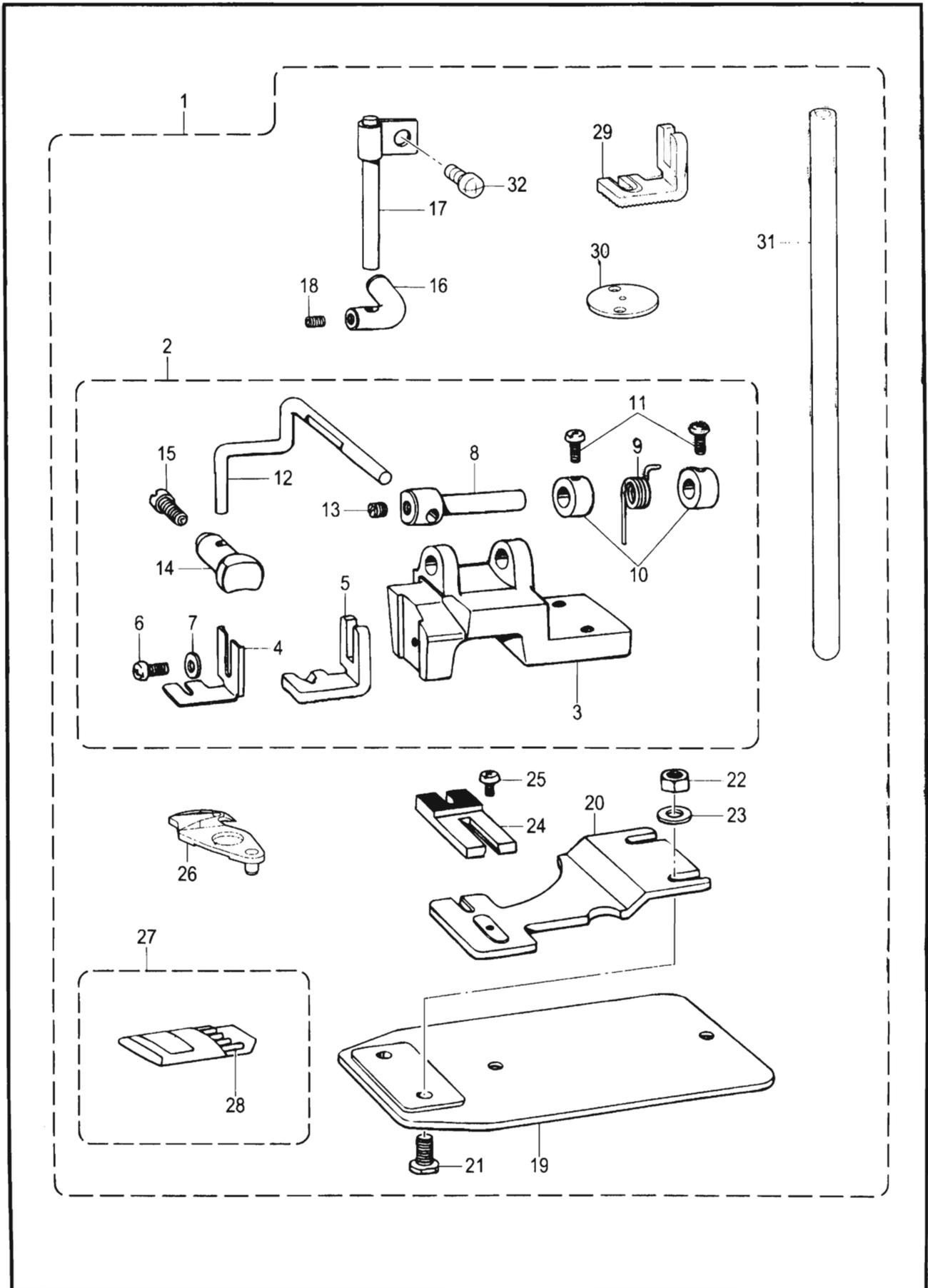
V1. 辅助装置(用于438D的选购零部件) / Auxiliary device (Option parts fo 438D )
