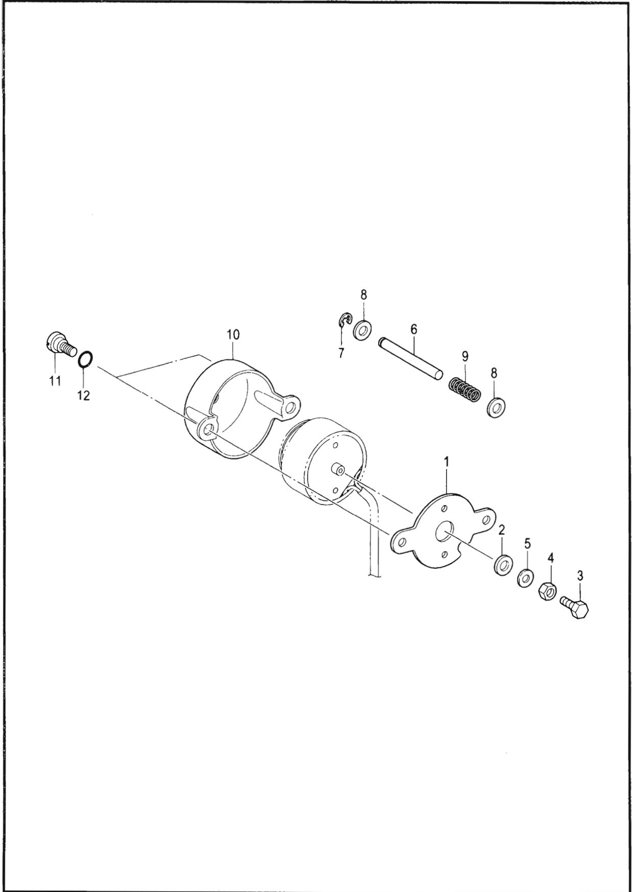
M. 系线装置 / Tension release mechanism
