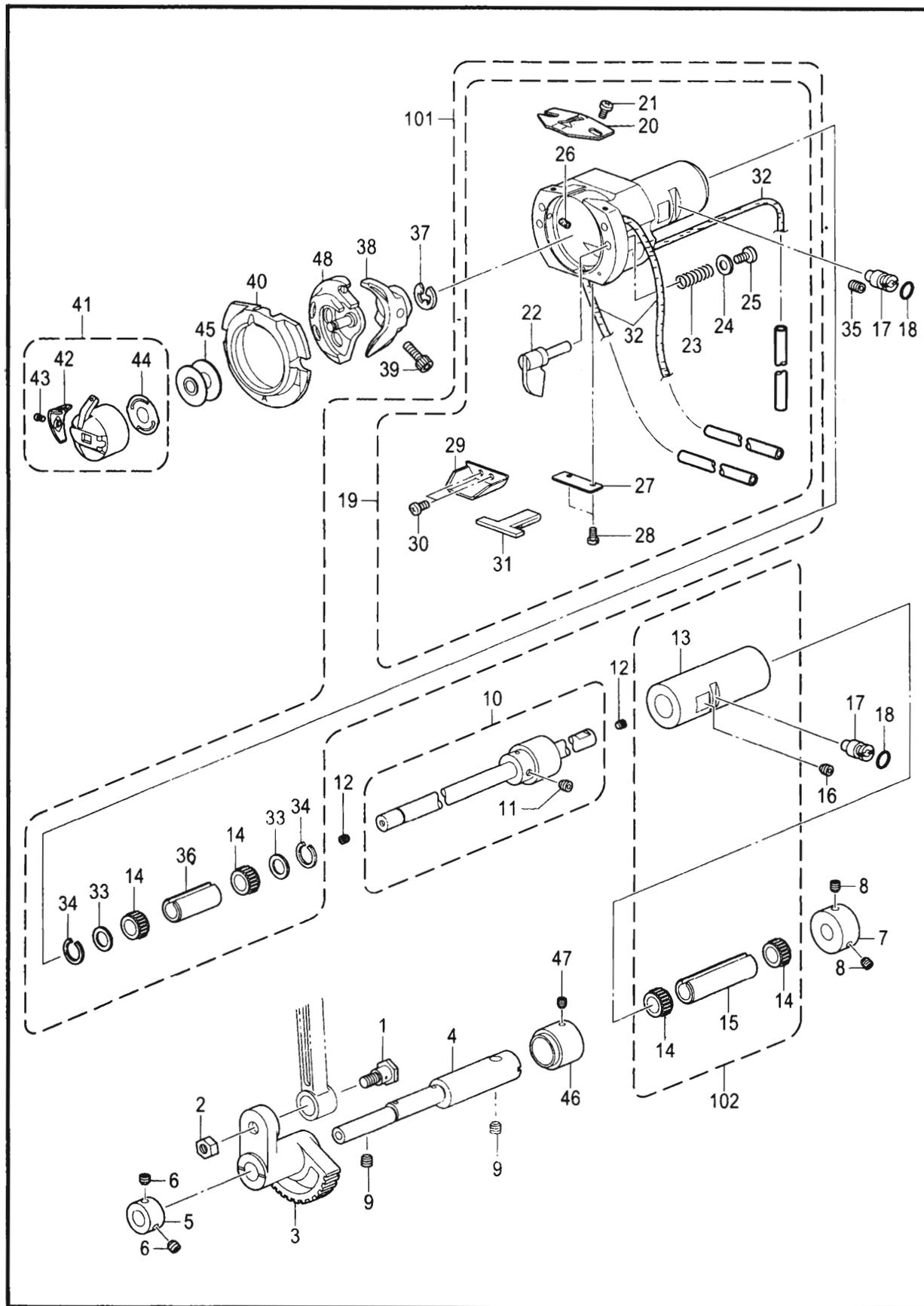
F. 下轴装置 / Lower shaft mechanism
