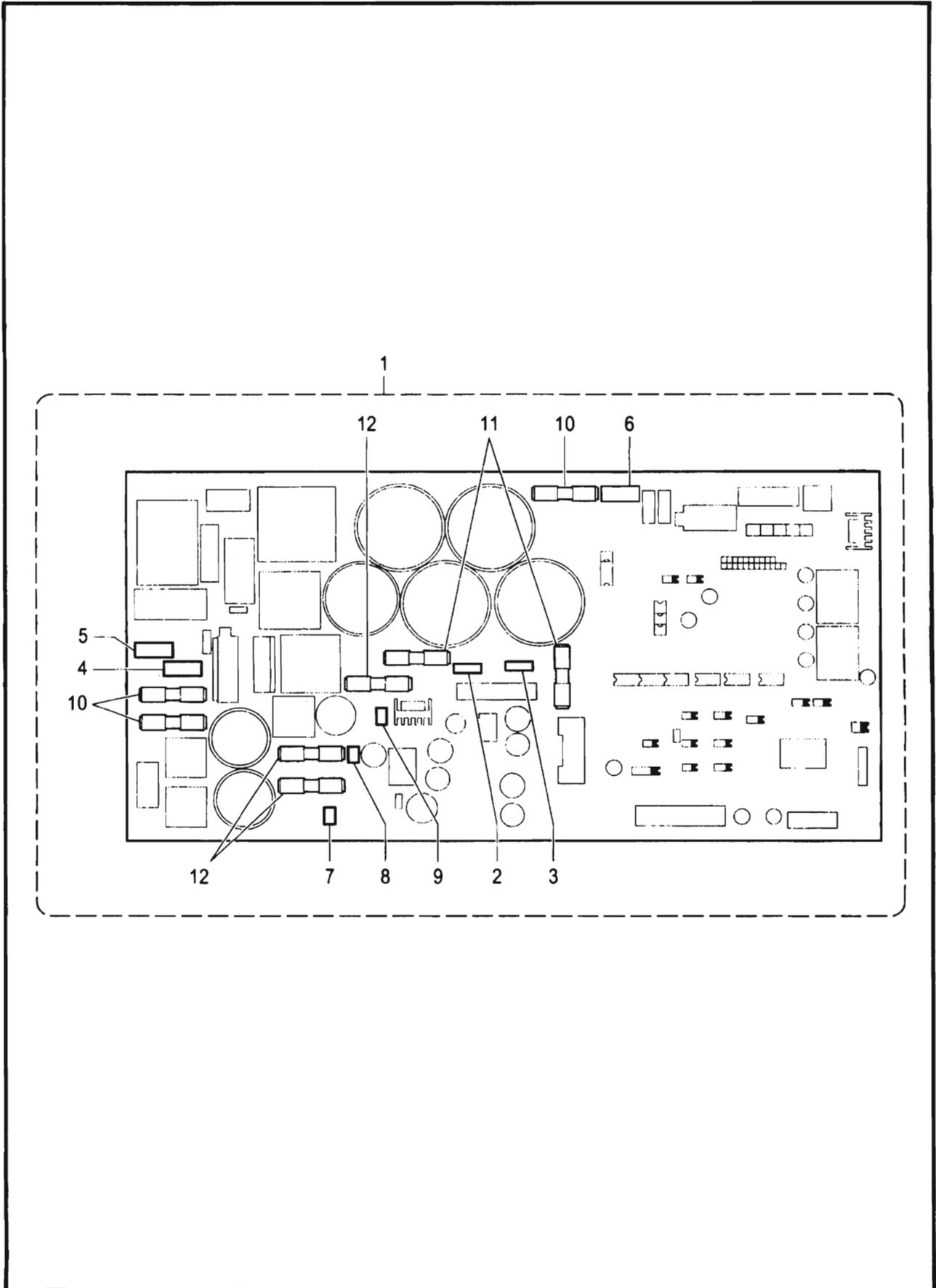
P2. 控制箱装置(电源基板) / Control box (PCB) mechanism
