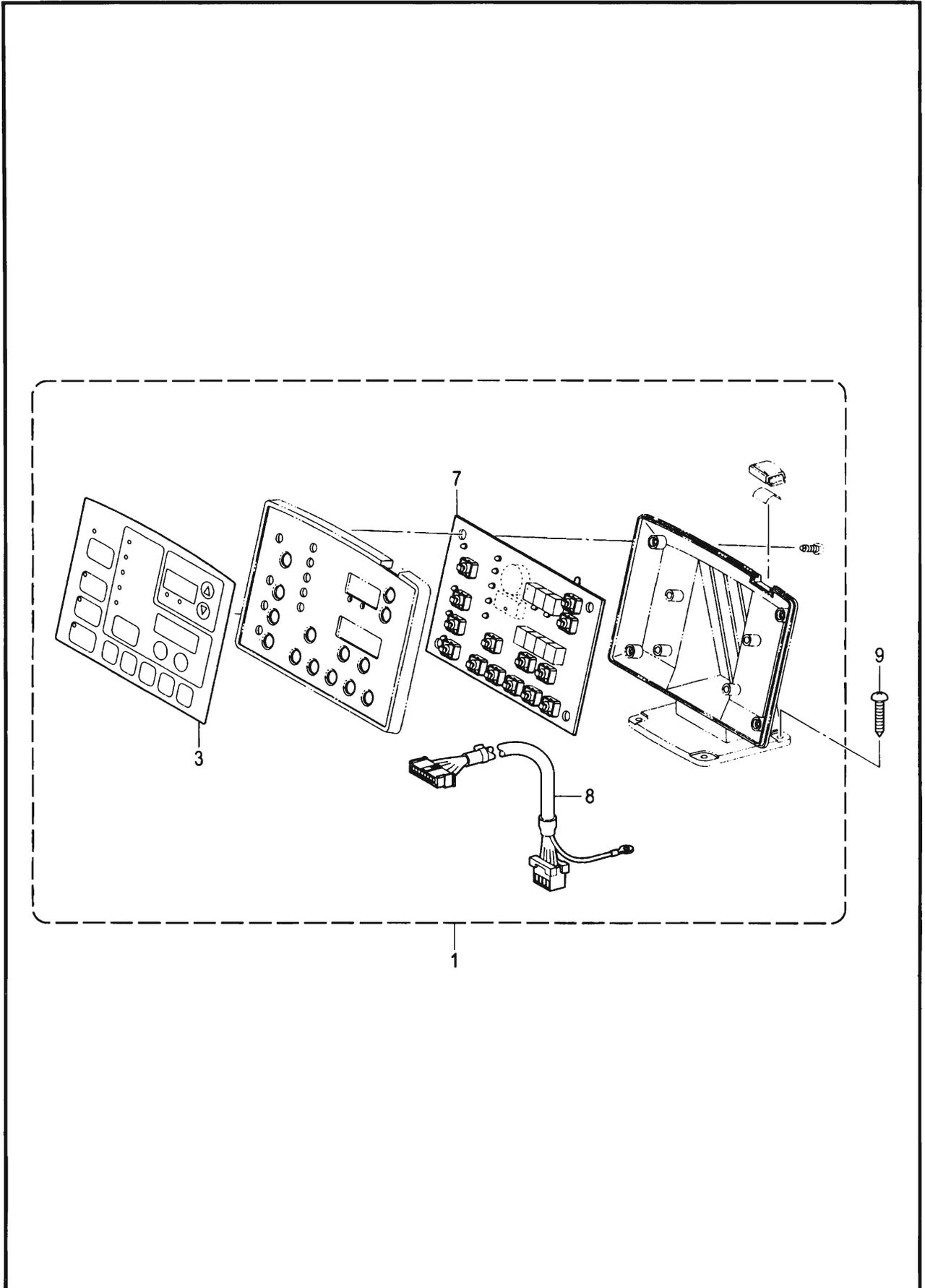
S. 操作盘装置 / Operation panel mechanism
