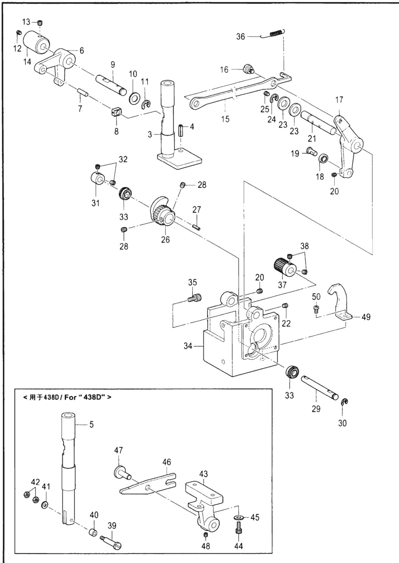
D. 抬压装置 / Work clamp lifter mechanism
