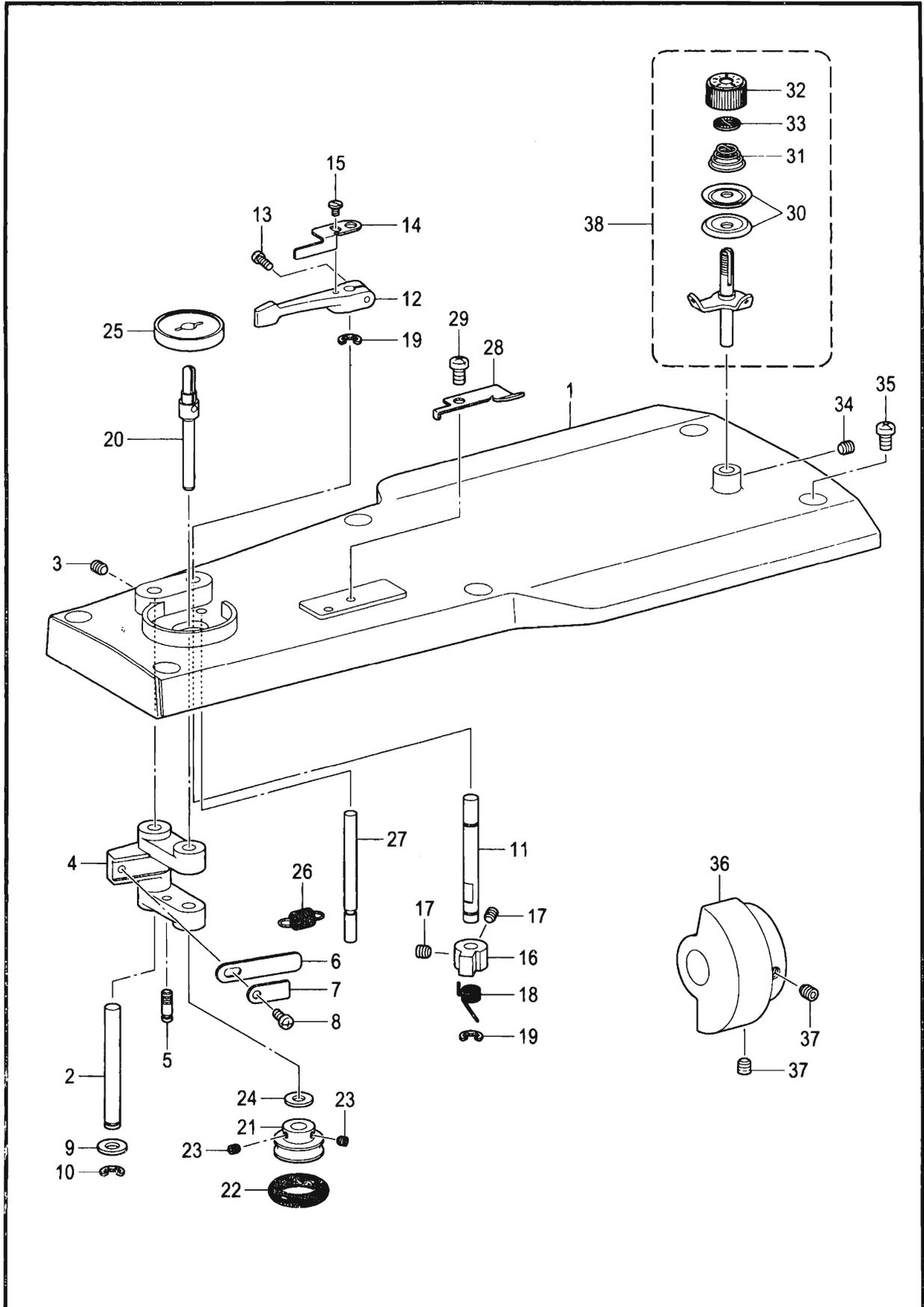
J. 卷线装置 / Bobbin winder mechanism
