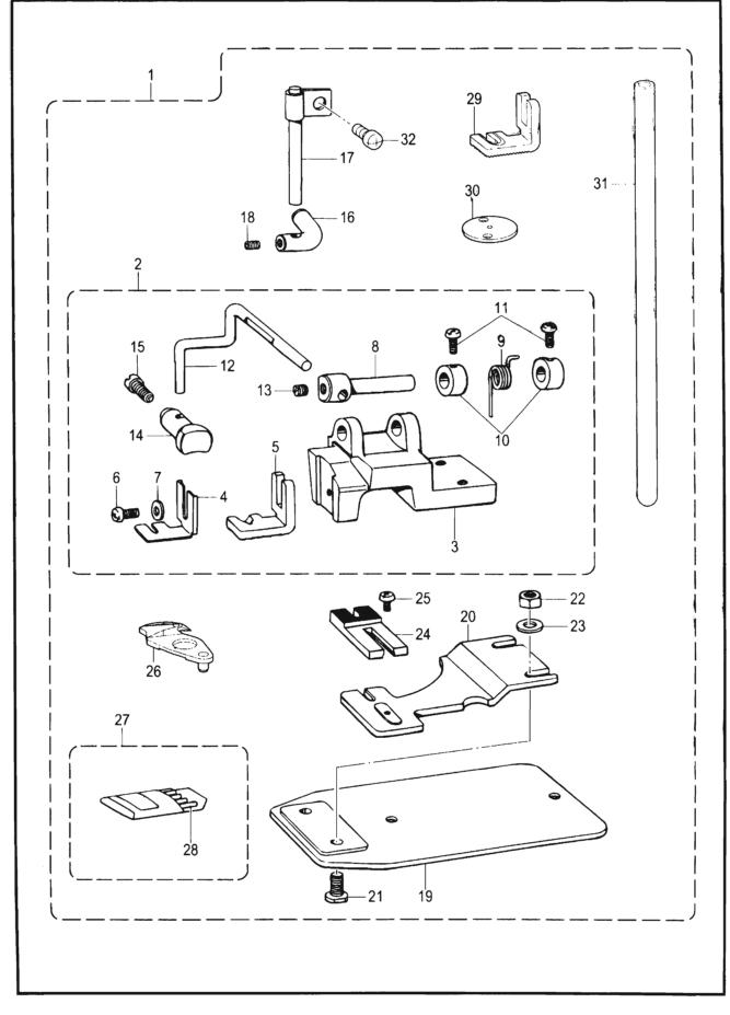
V1. 辅助装置(用于438D 的选购零部件) / Auxiliary device (Option parts for 438D)
