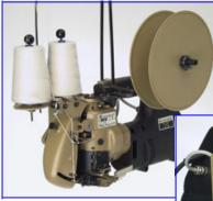
Sew-thru tape closure Styles 2200AB, BB come with tape folder and solenoid operated tape cutting device. Compressed air-powered Styles 2200L, LA are ideal for wet environments.
