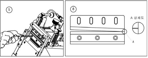
Mount of roll Fix the roll triangle by 4mm-wrench.
